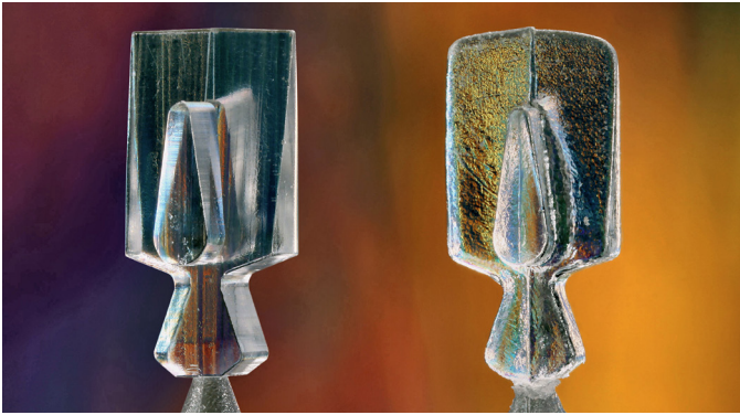
Major differences in quality and shape accuracy results between 3D Micro EDM Milling (right) and EDM-sinking (left)
