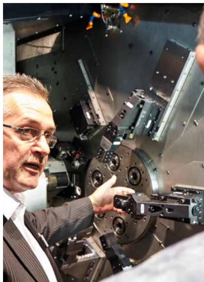
operation. Their superb ergonomics, incorporating front access and integrated peripherals, make setup a snap, and their simplified programming makes it easy for single-spindle operators to get great results. The machines ultra-dynamic and entirely independent spindles allow angular positioning and optimal speeds in each position. Since each spindle has its own Z axis with hydrostatic bearings, you get flawless finishes and extend the lifetime of your tools by 30 to 40 percent.
