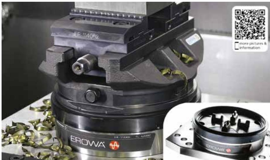
The 10,000N clamping power of the PowerChuck P guarantees a powerful and reliable grip for workpiece machining. The compact design and the low height of the tooling system leave a great deal of space for workpieces and their machining processes. The base plate of the PowerChuck P has a versatile mounting hole configuration, thus offering many fitting options.
