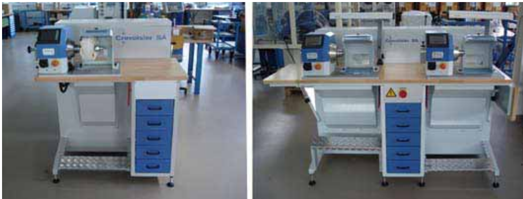
standard table grinding machines are compatible with ECO C5001 simple or double stand-alone working places. An integrating vacuum system complete these features.
