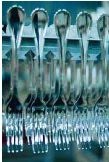
detergent baths in the final cleaning phase for our pieces. Today, when the question of replacing our inter-operational trichloroethylene installations arises, we have once again, after evaluation of the different options, chosen to use NGL Cleaning Technology baths. So, we can entirely eliminate solvents from our manufacturing process.
