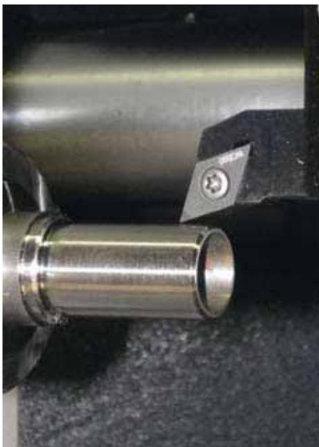
balance has been developed specifically to minimise dilation. It has a single spindle and particular care was taken in designing it. The circularity obtained during controlled tests was 0.18 µm. The numerical control uses ISO programming and has a resolution up to one-tenth of a micron. Tests show outstanding machining stability. For example, when
