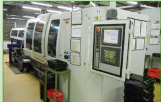
CNC Multispindle lathe TORNOS
