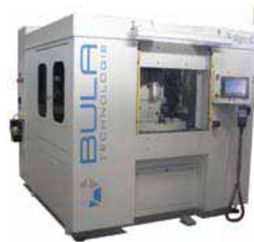
The new Beta 3 Poligo center of Bula Technologie allows polishing, colouring, brushing and deburring. Medical parts finishing is child's play.
