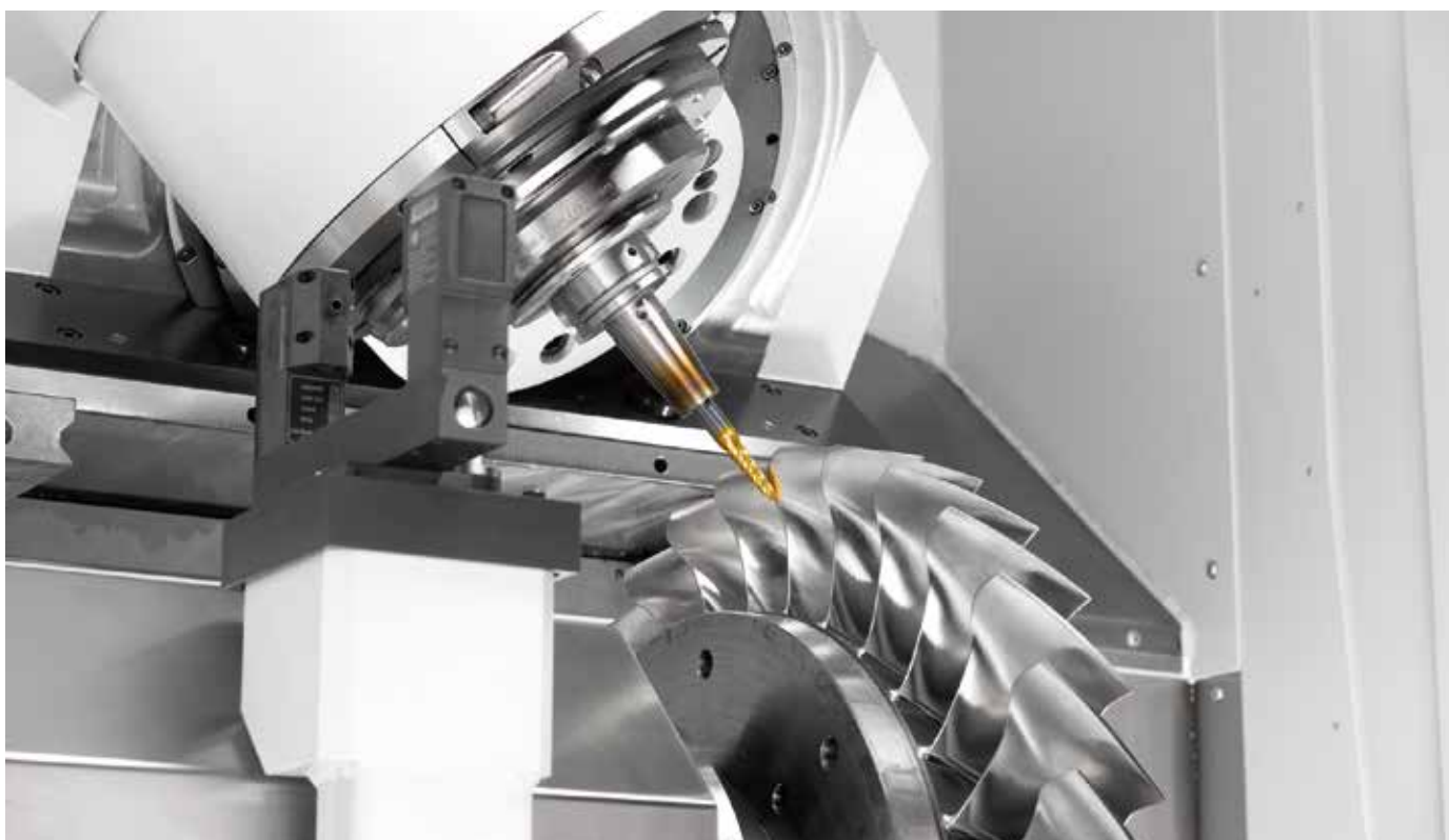
Usinage de composants de turbine. Zerspangung von Turbinenelementen. Machining of turbine components.
